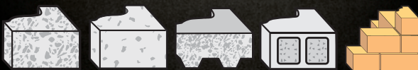
Normal Weight Concrete Light Weight Concrete Concrete Over Steel Deck Grouted Masonry Brick
