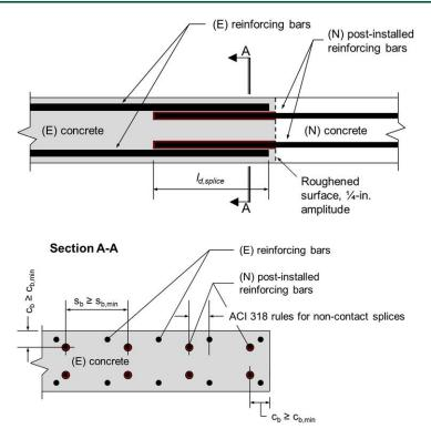
FIGURE 2—INSTALLATION PARAMATERS FOR POST-INSTALLED REINFORCING BARS
