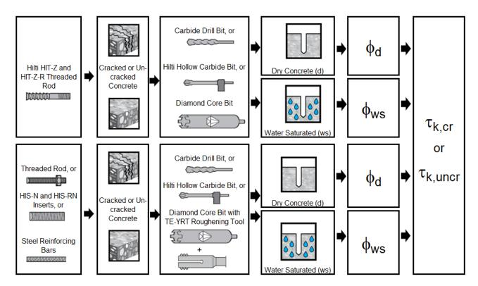
FIGURE 4—FLOWCHART FOR THE ESTABLISHMENT OF DESIGN BOND OR PULLOUT STRENGTH FOR POST-INSTALLED ADHESIVE ANCHORS
