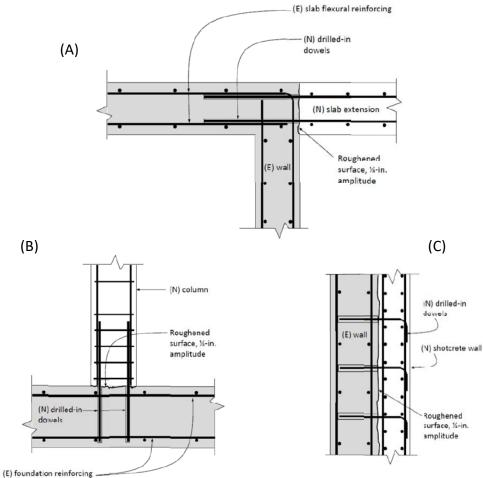
FIGURE 3—APPLICATION EXAMPLES FOR POST-INSTALLED REINFORCING BARS:
