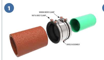
Loosen bolts on stainless steel shield assembly (worm drive clamps) and end clamps (Nut & Bolt). Do not remove the shield assembly or end clamps from the gasket.
