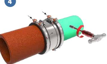
Tighten Nut & Bolt clamps alternately and firmly to 60 in/lbs. of torque.
