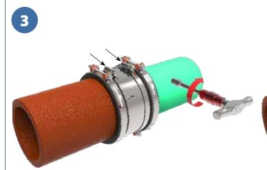
Tighten worm drive clamps alternately and firmly to 60 in/lbs. of torque.
