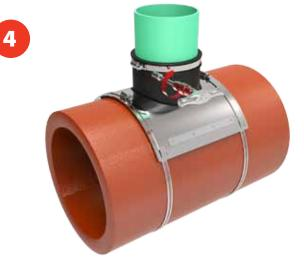
Loosen lateral inlet worm drive clamp. Insert lateral pipe into mouth of inlet until it rests against the internal pipe stop. Tighten lateral inlet worm drive clamp to 60 in/lbs. of torque.
