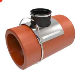
Core appropriate sized hole into sewer main (4" core i.d. of 4.60" - 4.90" & 6" core i.d. of 6.60" - 6.90"). After making sure pipe surface is clean and free of debris, wrap stainless steel apron and gasket around sewer main, making sure internal flange of gasket is centered in hole of cored pipe.
