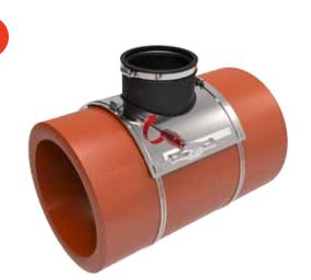
Pull screw head away from clamp housing and pull "tail" through housing. Cinch down clamp to hand-tight. Note: Housing should be centered onto apron. Repeat clamp installation on opposite side. Using a nut driver or torque wrench, tighten quick-release clamps alternately and firmly to 60 in/lbs. of torque. Slide clamp "tail" back through top of square eyelet.
