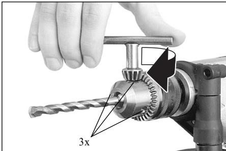
**Chucking the tool:** Insert the tool and use the chuck key to uniformly clamp tight all 3 bores.
