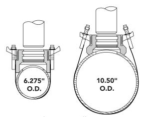
Same saddle conforming to different outside diameters.
