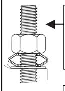
Smith-Blair® Belleville Washers (p/n 150115-000) must be used on PE pipe installations. Use of any other type of Spring Washer may cause product failure.
