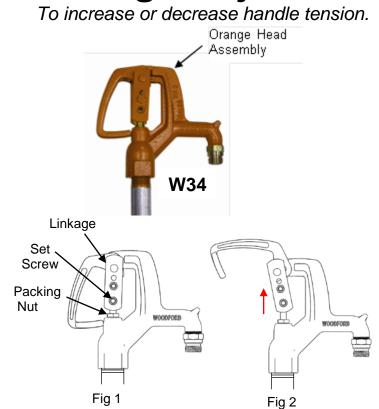
If the Handle does not "snap" closed approximately 3" from the head casting upon turning off the hydrant, follow the instructions to adjust the linkage and handle tension.
