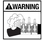
THIS PRODUCT DOES NOT RESTRAIN PIPE MOVEMENT. Proper anchoring is required to prevent pipe pull out. Failure to anchor or improper anchoring can result in dangerous pipe content escape, property damage, serious injury, or death. Refer to smith-blair.com for products designed to restrain axial pipe movement. Read the product installation instructions prior to installing this product.
